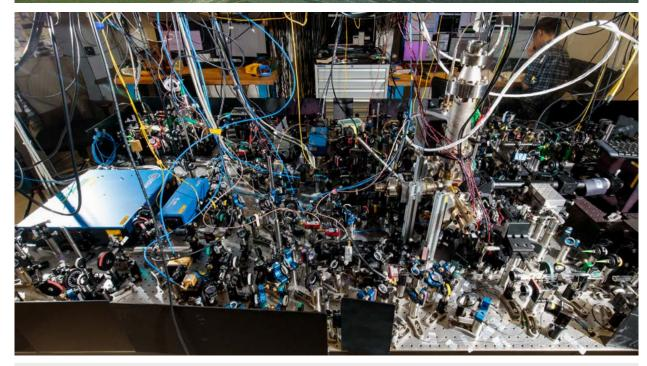
To perform experiments in continuous variable quantum computing, the group uses this entire setup. It occupies a table measuring 4m x 1.5m. In total, there are about 400 to 500 optical elements such as mirrors and lenses.
