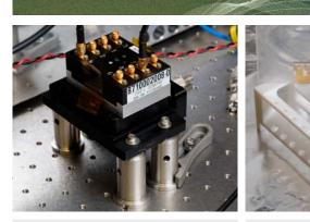
The group is making upgrades to their experiment, including adding an acousto-optical modulator with eight channels. This can direct eight laser beams, so the group will be able to control eight ions simultaneously. The team's old modulator only had a single channel.
