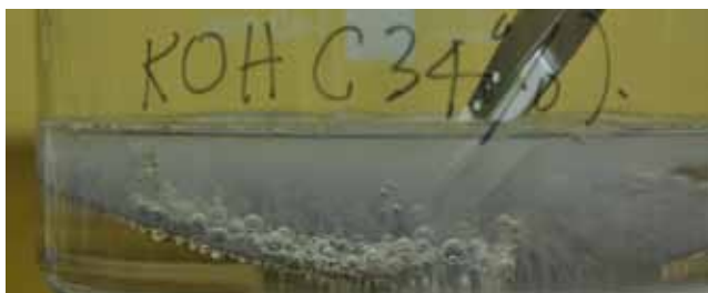
▲ Figure 3: (Top) Don't try this at home! (Bottom) A diamond-coated silicon wafer is boiled in potassium hydroxide to remove the silicon. When the silicon is removed, we are left with wires supported by a diamond film.
