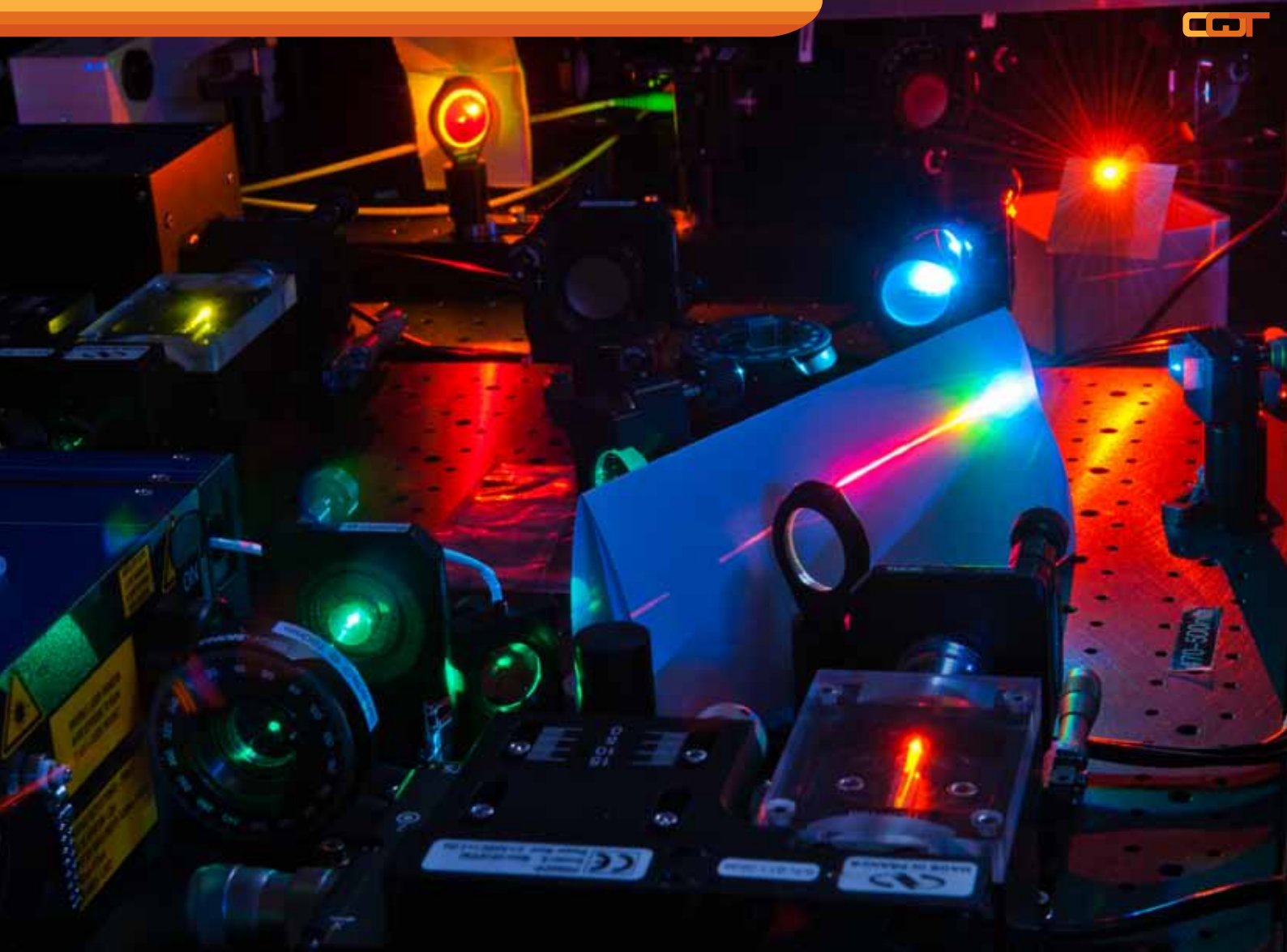
▲ The rainbow of light produced by the frequency comb is made of millions of sharply-defined lines of colour.
