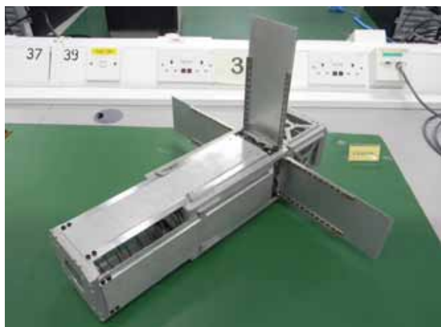
◀ Figure 2: CQT is teaming up with the Satellite Research Centre at Nanyang Technical University, which plans to launch the 3U Velox-I (pictured). This a 3U CubeSat, the size of three 1U CubeSats, that will separate into a 2U and 1U section to test communication technologies between the free-flying sub-units. The CQT experiment will occupy a 3cm-thick section of the 1U unit located above the solar panel holders.
